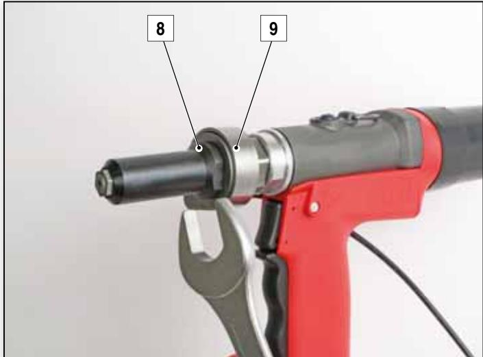
To reveal the signal precisely, be sure that the sleeve (**8**) of the riveting tool is correctly fixed against the sensor (**9**).
